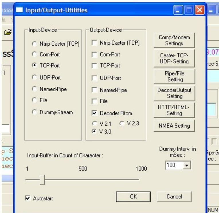
From the Input-Device menu choose TCP-Port. From the Output-Device menu choose Decoder RtcM V3.0
